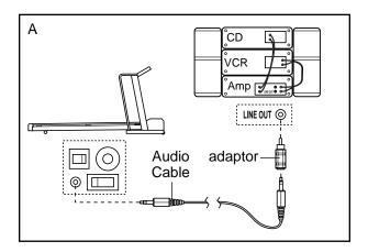
B. Plug one end of the audio cable into the jack on the front of the treadmill near the power cord. Plug the other end of the cable into the included adaptor. Plug the adaptor into an RCA Y-adaptor (available at electronics stores). Next, remove the wire that is currently plugged into the LINE OUT jack on your stereo and plug the wire into the unused side of the RCA Y-adaptor. Plug the RCA Y-adaptor into the LINE OUT jack on your stereo.
